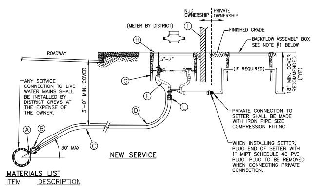
A DIRECT TAP: DIRECT TAP OF DUCTILE IRON OR CAST IRON LARGER THAN 4" DIAMETER IS REQUIRED FOR 1" SERVICES. SADDLES WILL NOT BE ALLOWED ON DUCTILE IRON OR CAST IRON PIPE LARGER THAN 4" DIAMETER.
